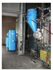
The 1020MFS shown to the left is being used to reclaim Steel Shot and introduce it back into the customer's shot blast machine via a VAC-U-MAX Intercept Hopper.
