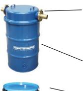
MDL 115-01 Heavy-duty Intercept Cover assembly for 55 gallon drums, complete with replaceable stainless steel inlet and outlet adaptors, internal impact baffle plate with replaceable rubber absorption flap, neoprene gasket with grounding strap, lifting handles, and carbon steel construction with blue powder coat finish.
