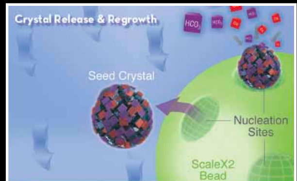
Once the crystals grow to a certain size they are released from the bead. The crystals in solution keep the hardness out of the water so that it can't form scale or interfere with soap.
