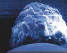
Once the crystals grow to a certain size they are released from the bead. The crystals in solution keep the hardness out of the water so that it can't form scale or interfere with soap.
