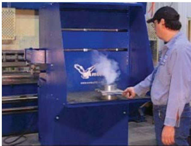
Removes Contaminates from the Breathing Area of the Operator.
